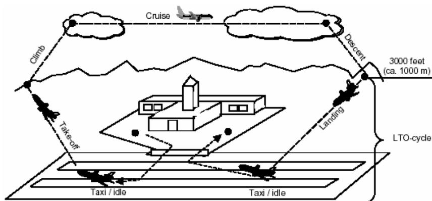
Figure 1. Phases of flight of aircraft<sup>4</sup>
